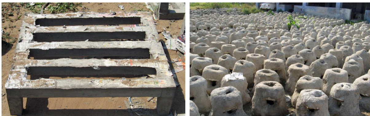
FIGURE 5: CONCRETE FRAME (LEFT) AND FISH HOUSE (RIGHT) USED TO CONSTRUCT ARTIFICIAL REEFS
